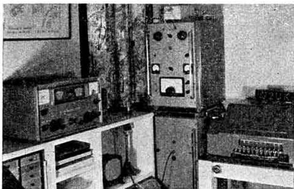
G2UK's RTTY station. The transmitter is a LG300 modified for f.s.k. and the receiver is a Hammarlund HQ110. The teleprinter is a Creed Type 3, which has been replaced by a Teletype Model 14 since the photograph was taken. The f.s.k. receiving adaptor, which is only partially visible and is located in a rack below the monitor speaker shown, is a surplus commercial unit, Type A.P. 66862.
