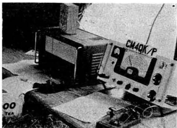
At Ayrshire Group's B station, GM4QK/P, the equipment included an Eddystone 888A receiver, a home-built transmitter employing a Geloso v.f.o. and dipoles for 20 and 40m.
