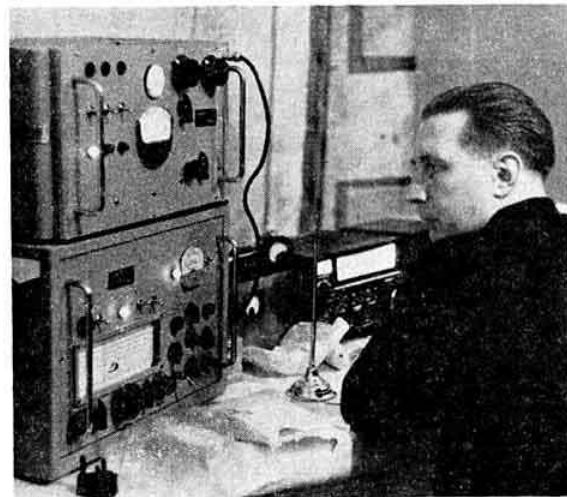
G3PED operating the single sideband h.f. station GB3DTS at the Dagenham Town Show. The transmitter was constructed by G3MYV.
